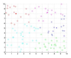
Fig. 2. Clustering of 100 2-d observations in five clusters using the k-means algorithm.
