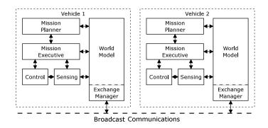
Fig. 3. The distributed world model architecture.
