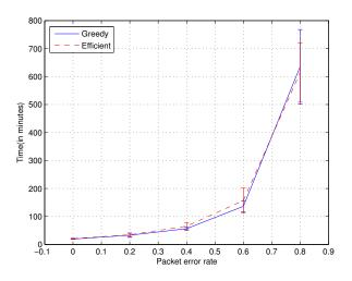
Fig. 4. Average mission completion time for different values of packet error rate.
